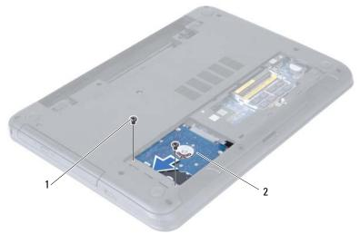
screws (2) hard-drive assembly **3** Using the pull-tab, lift the hard-drive assembly out of the computer base.
